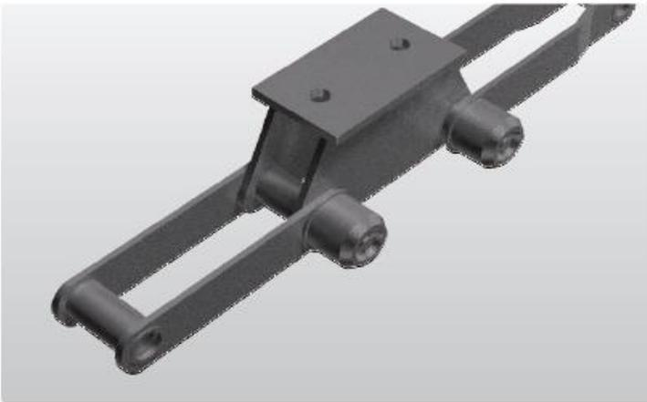
When abrasive material infiltrates between bushes and rollers, and infiltrates outboard rollers, the rollers lock and wear accelerates between bush and roller, causing your chain to reach its wear life. Using TSUBAKI's dust resistant bearing rollers extends the life of your reclaimer chain.
